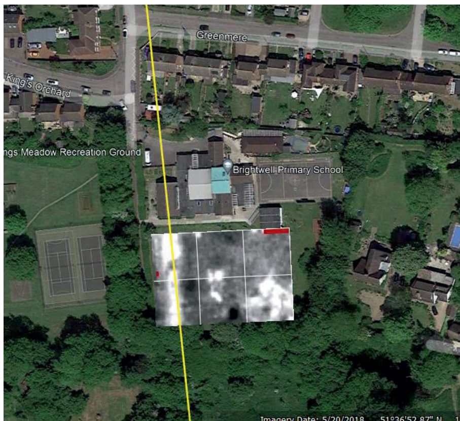
Figure 32: The route of the Silchester–Dorchester–Alchester Roman road (yellow line) and the results of the resistivity survey
